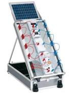
Carrying out current and voltage measurements with a solar energy kit to create a characteristic curve with its maximum power point and compare provided examples.
